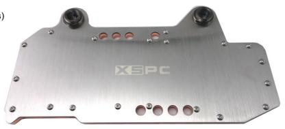
**Note:** This waterblock is only suitable for reference design GTX590 cards. If you are unsure if your card if a reference design GTX590 contact us prior to installation to make sure.
