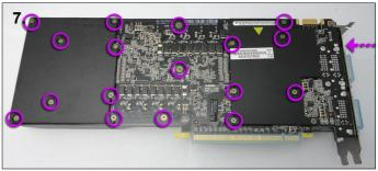
**7.** Remove the two screws on the bracket next to the DVI ports. Now turn the card on its back and remove the 17 screws highlighted above.
