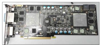
**9.** Clean the thermal paste from the GPU cores and chipset, ready for installation. Remove any residue left from the thermal pads.
