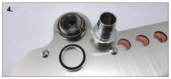
**4.** If you are using G1/4" barbs/fittings with a long thread you will need to use the supplied rings to avoid blocking the flow. Attach the barbs to your chosen ports using an adjustable spanner. Make sure the o-rings are fully compressed.
