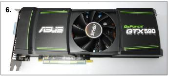
**6**. Before handing the card you should take precautions to avoid static damage. Remove the GTX590 card from the box ready for installation.
