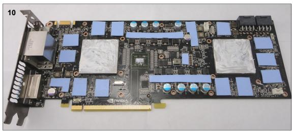
**10**. Remove the tape from both sides of the thermal pads. Place the blue pads on positions shown above. Next apply thermal paste to the GPU cores and chipset.
