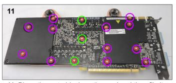
11. Place the waterblock on the card and then filp it over to line up the screw holes. Make sure the thermal pads stay in place. Now use twelve 8mm screws (marked in pink) and washers to attach the waterblock through the backplates. Finally use the three 6mm screws and washers on the holes in the middle of the PCB (marked in green).
