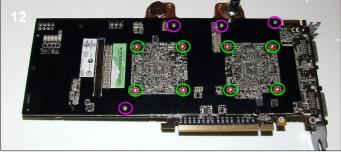
**12**. Finally use the 12 screws and 8 washers to attach the waterblock to the card. It is best to start with the 8 short screws and washers (green) around the GPU cores followed by the 4 long screws (pink) on the outer holes. Do not over tighten the screws as this may bend the card and cause damage.
