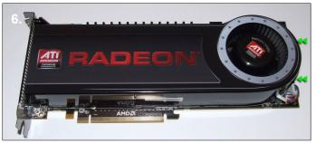
**6**. Before handing the card you should take precautions to avoid static damage. Remove the 4870X2 card from the box and unscrew the two screws to the right of the fan.
