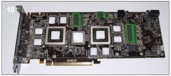
**10**. Remove the tape from both sides of the thermal pads and place them on the 6 locations marked in the photo above. Next apply thermal paste to the memory chips, chipset and the GPU cores.
