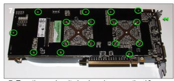
**7.** Turn the card on its back and remove the 16 screws highlighted above and the 2 screws near the DVI ports.
