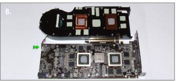
**8**. Turn the card back over and carefully remove the heatsink and fan, leaving the ATI backplate on the card. Now the card and heatsink are separated detach the fan power cable from the fan header.
