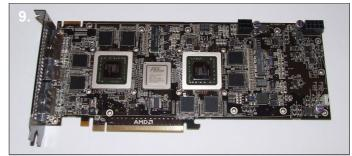
**9.** Clean the thermal paste from the GPU cores ready for installation. Remove any residue left from the thermal pads.
