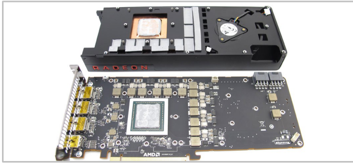
6. Turn the card back over and carefully remove the heat sink and fan. Now the card and heat sink are separated detach the fan power cable from the fan header.
