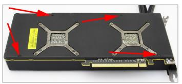
7. Turn the card on its back and remove the 4 screws highlighted in red. Now remove the backplate.
