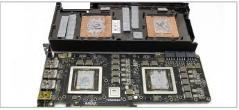
9. Carefully remove the heat sink and detach the power cables from the power headers.
