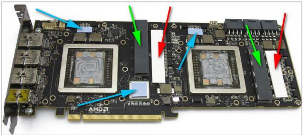
11. Remove the tape from both sides of the thermal pads. Place the 1.5mm pads in the positions marked in red, the 1mm pads in the positions marked in blue, and the 0.5mm pads in the positions marked in green. Now apply thermal paste to the GPU cores and memory stacks.
