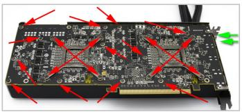
**8.** Remove the 20 screws highlighted in red and the two screws marked in green from the i/o bracket.
