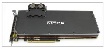
13. The card is now ready for use. When you first boot it is advisable to use software to check the core temperature. If the temperature is high you will need to remount the block.
