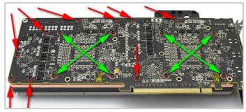
12. Place the waterblock on the card to line up the screw holes and then flip it over (make sure the thermal pads stay in place). Fit the provided screw and washers to the positions marked above. It's best to fit the screws marked in green first. Tighten each screw gradually to make sure equal pressure is applied. Over tightening can permanently damage the card.
