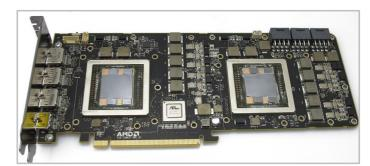
10. Clean the thermal paste from the GPU cores and memory stacks with a soft cloth. Do not attempt to clean any paste left between the core and memory stacks, as this can cause damage.
