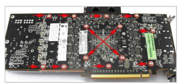
11. Place the waterblock on the card to line up the screw holes and then flip it over - making sure the thermal pads stay in place. Now carefully attach the block to the card using the supplied screws and washers. You should start with the four holes behind the GPU and gradually tighten each screw.
