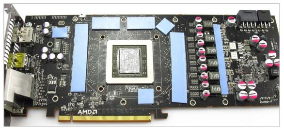
10. Remove the tape from both sides of the thermal pads. Place the blue pads on the eight positions shown above and finally apply thermal paste to the GPU core.
