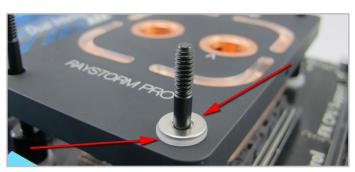
4. Place a plastic washer and metal washer over each of the four posts.
