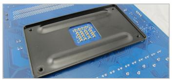
2. If the backplate is loose, place it back in its correct position. Make sure the 4 screw threads on the backplate line up with the holes on the motherboard.
