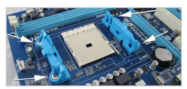
1. Remove the plastic clips on either side of the CPU socket by undoing the 4 screws.
