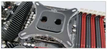
3. Place the waterblock onto the CPU and line-up the mounting plate with the holes on the motherboard.
