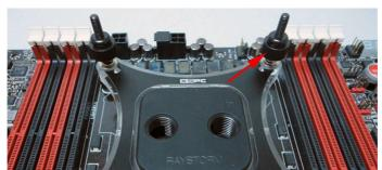
Place a nut over each post and gradually tighten them. Make sure to apply equal pressure to each spring.
