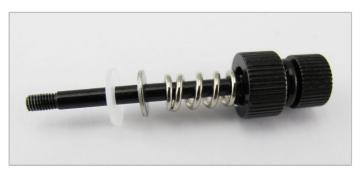
4. Place a spring and washers over each bolt. Bolt >Nut >Spring >Metal washer >Plastic Washer
