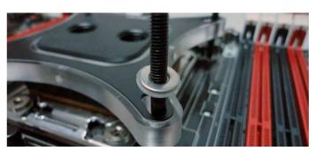
4. Place a plastic washer and metal washer over each of the four posts.
