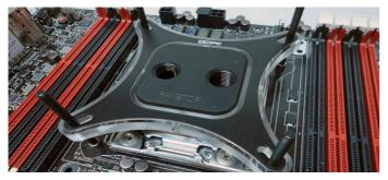
3. Place the waterblock over the M4 posts and onto the CPU.
