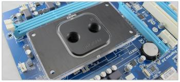
3. Place the waterblock onto the CPU and line-up the mounting plate with the holes on the motherboard.
