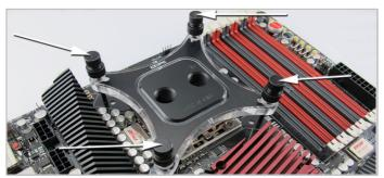
5. Place each of the bolts through the mounting plate and loosely screw into the backplate using the knurled section of the bolt [A]. When all 4 bolts are loosely fitted, tighten each bolt [A].
