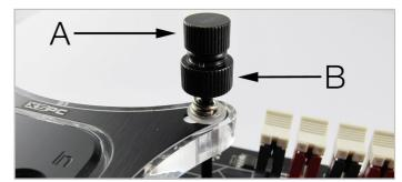
6. Use the lower knurled nut [B] to adjust the pressure on the CPU. Make sure to apply equal pressure to each spring.
