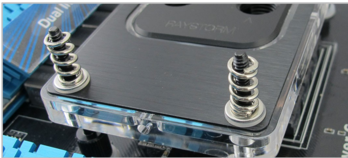
5. Place a spring over each of the four posts.
