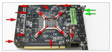
7. Turn the card on its back and remove the 13 screws highlighted in red and the two screws marked in green from the i/o bracket.
