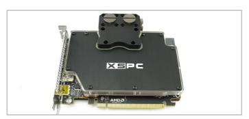
12. The card is now ready for use. When you first boot it is advisable to use software to check the core temperature. If the temperature is high you will need to remount the block.
