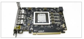
**8**. Carefully remove the heat sink and detach the power cable from the power header.
