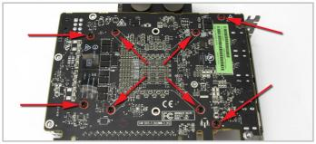
11. Place the waterblock on the card to line up the screw holes and then flip it over (make sure the thermal pads stay in place). Fit the provided screw and washers to the positions marked above. Do not over tighten the screws as this may bend the card and cause permanent damage.
