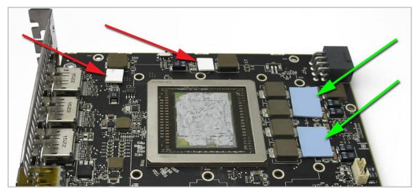
10. Remove the tape from both sides of the thermal pads. Place the 1.5mm pads in the positions marked in red, and the 1mm pads in the positions marked in green. Now apply thermal paste to the GPU core and memory stacks.
