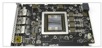
9. Clean the thermal paste from the GPU core and memory stacks with a soft cloth. Do not attempt to clean any paste left between the core and memory stacks, as this can cause damage.
