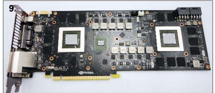
**9.** Clean the thermal paste from the GPU cores, chipset and remove any residue left from the thermal pads.
