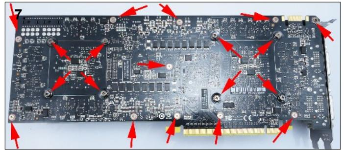
**7.** Now turn the card on its back and remove the 19 screws highlighted above.
