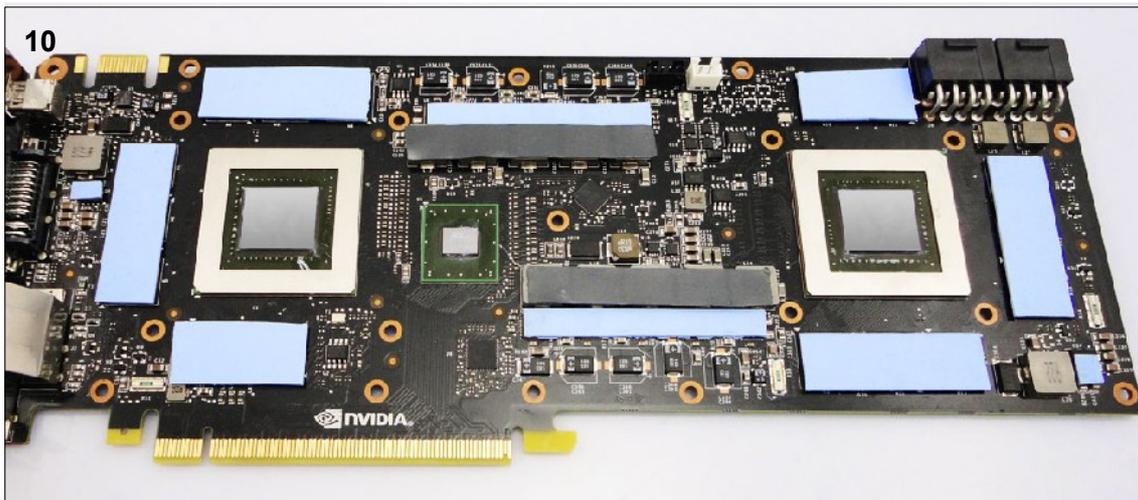
**10.** Remove the tape from both sides of the thermal pads. Place the ten blue pads and two grey pads on the positions shown above. Next apply thermal paste to the GPU cores and chipset.
