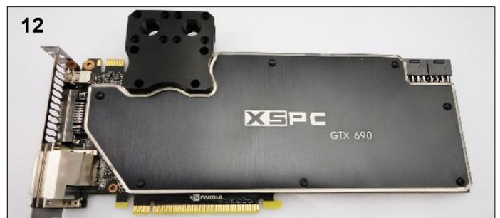
**12.** Do not over tighten the screws as this may bend the card and cause permanent damage. The card is now ready for use. When you first boot it is advisable to use ATITool or other monitoring software to check the core temperature. If the temperature is high you will need to remount the block.
