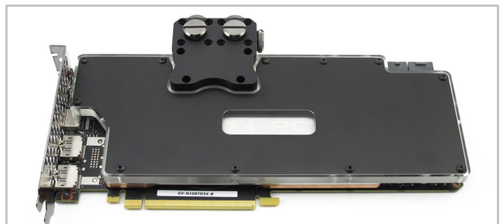
13. Do not over tighten the screws as this may bend the card and cause permanent damage. The card is now ready for use. When you first boot it is advisable to use software to check the core temperature. If the temperature is high you will need to remount the block.
