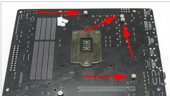
1. Turn the board over and remove the four screws highlighted above. Keep these to one side, they will be needed in step 5.
