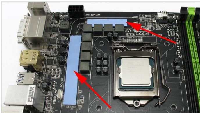
3. Remove the film from both sides and place the blue thermal pads on the positions marked above.
