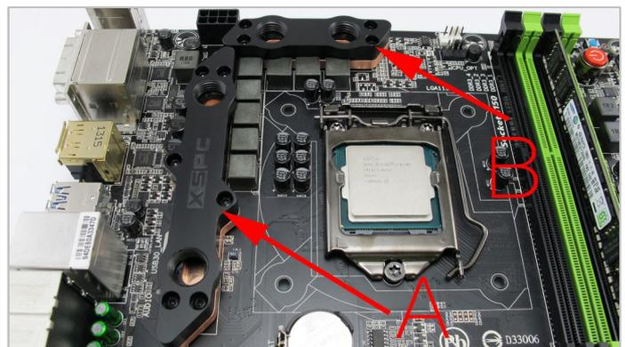
4. Remove the plastic film from the A and B water blocks and carefully place them into position on the motherboard. You should check the thermal pads are still in position.
