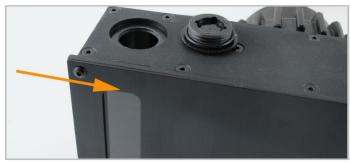
7. With the fill cap removed fill the reservoir with coolant until it reaches just above the top of the coolant level window. You will have to keep topping up the reservoir as the air bleeds from the loop.
