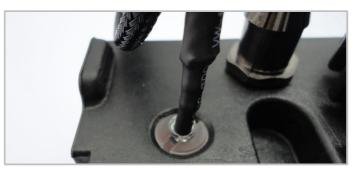
5. Push the 5mm LED into the acrylic cap to provide a backlight to the coolant level window.
