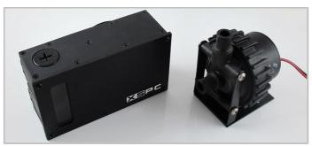
1. Installation requires the D5's screw ring. First turn the screw ring anti-clockwise to remove the front of the D5 pump and o-ring.
