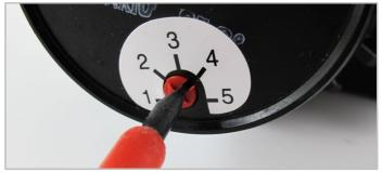
8. The dial on the back of the pump can be used to set the pump speed. 5 being full power and 1 being the lowest noise level.
