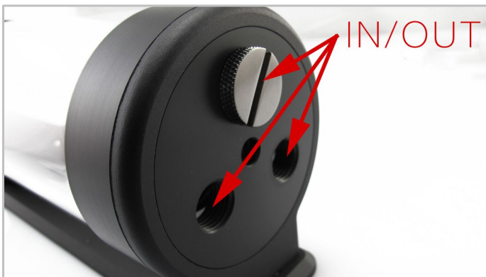
3. The reservoir has three G1/4" ports on the base. All of these can be used as either an inlet or outlet. Attach the hose fittings to your ports of choice.
