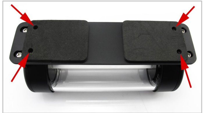
2. Stick the pads to the back of the reservoirs bracket. Make sure the screw holes on the bracket line up with the holes on the pads..
