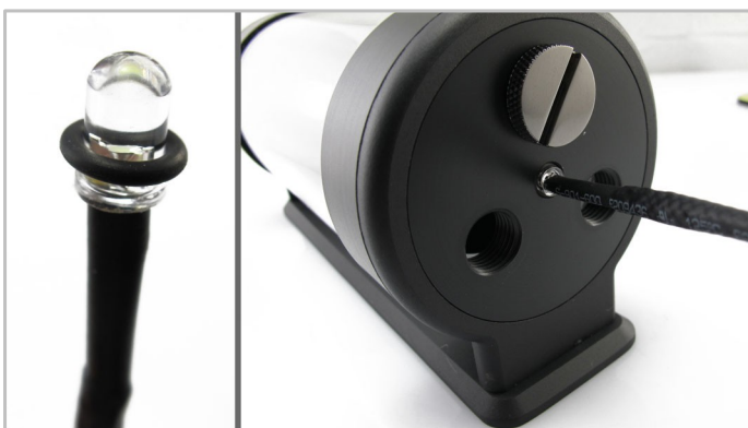
5. Place the o-ring over the LED and push it into the hole on the base of the reservoir.
