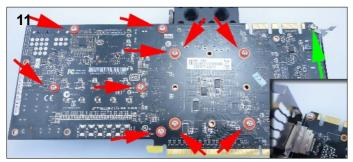
**11.** Place the waterblock on the card to line up the screw holes and then filp it over, making sure the thermal pads stay in place. Now carefully attach the block to the card, starting with the four holes behind the GPU. The screw marked in green requires an M3 nut attaching on the other side of the card.
