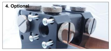
**4.** If you are using cards in SLI you can use the optional SLI flow connector to bridge the two cards. This should be done after step 12.
