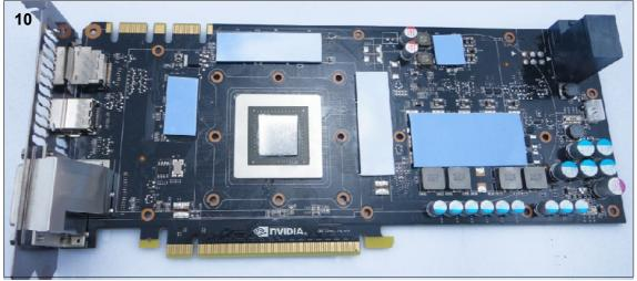
**10**. Remove the tape from both sides of the thermal pads. Place the blue pads on the five positions shown above. Next apply thermal paste to the GPU core.
