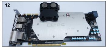
**12**. Do not over tighten the screws as this may bend the card and cause permanent damage. The card is now ready for use. When you first boot it is advisable to use ATItool or other software to check the core temperature. If the temperature is high you will need to remount the block.
